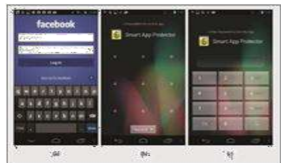
Fig 2: Different types of passcodes: a) Password; b) Pattern; c) PIN
