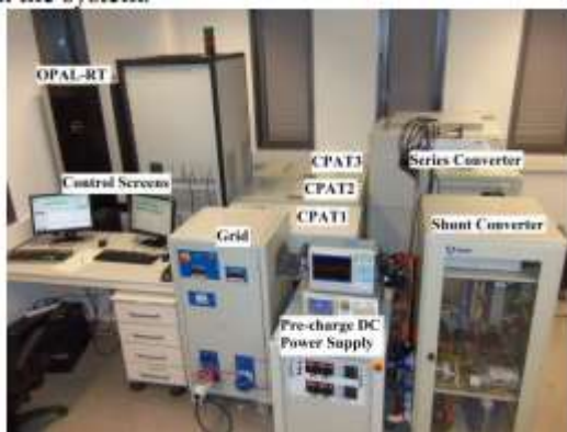
Fig. 16. Laboratory setup layout of the three-phase CPAT-UPFC
