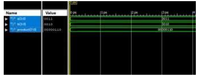
Fig. 4.Simulation Output of Vedic Multiplier
